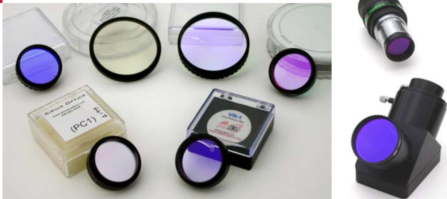
TAKING THE FRINGE OUT Filters specially designed to reduce the effects of chromatic aberration in achromatic telescopes thread into a diagonal or into the base of an eyepiece (right). The six filters we tested are, clockwise from upper left, Celestron-Baader, Lumicon, Baader, Orion, William Optics and Sirius Optics.
